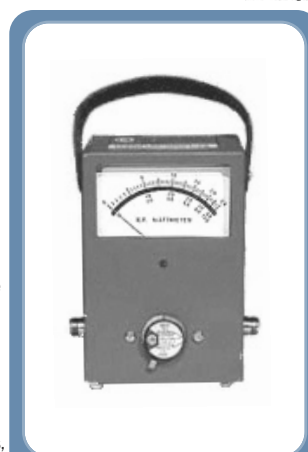
Shock mounted "taut band" Meter
