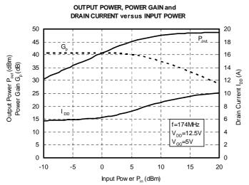
RoHS Compliance ,136-174MHz 60W 12.5V, 2 Stage Amp. For MOBILE RADIO
