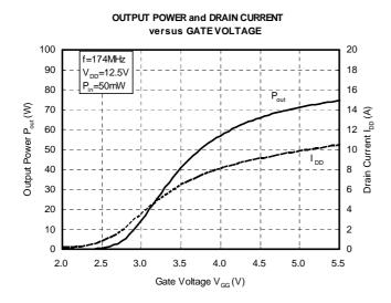
RoHS Compliance ,136-174MHz 60W 12.5V, 2 Stage Amp. For MOBILE RADIO
