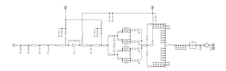
RoHS Compliance ,136-174MHz 60W 12.5V, 2 Stage Amp. For MOBILE RADIO
