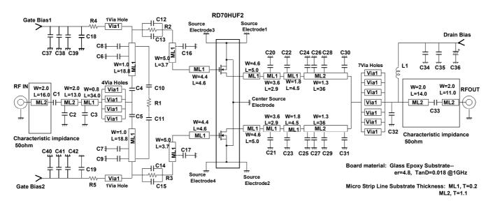
Via Hole Dimensions, Diameter=0.8 Length=1.6
