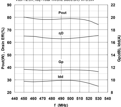
RoHS Compliance, Silicon MOSFET Power Transistor, 175MHz, 530MHz, 70W
