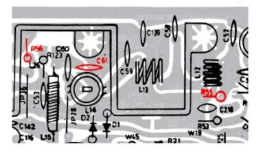
2) Install EKL Components' EN-1230 at R56. The EN-1230 is a POLARIZED part. Make sure that it is installed correctly with the positive lead toward R123.
