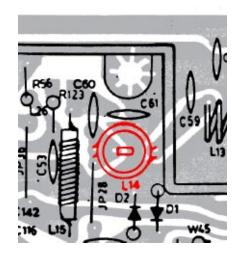
5) Remove TR14 (the 2SC2078), and install EKL Components' ERF-2030 in its place with stock insulator, washer, and screw.
