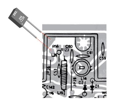
3) Add 68pF capacitor on back of C59. Install on solder side of PCB. Leave C59 capacitor alone.
