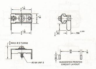
Style "B" - This capacitor style is supplied with a raised staple and solid terminals for printed circuit application.
