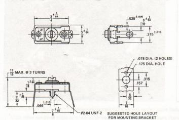
**Style** "A" — This capacitor style is supplied with a staple which is used for mounting the trimmer on a 5/16" width bracket. The capacitor terminals have elongated holes for point to point wiring.
