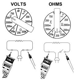
For DC Volts, set the meter to DC Volts instead of AC Volts.
